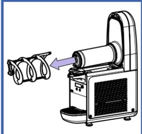
2. Remove the outer magnetic rotor assembly. The assembly is secured to the evaporator by a magnet and may need sufficient force to break the magnetic field.
