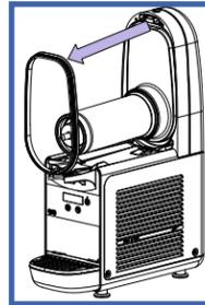
4. Remove the spigot pin and pull the spigot assembly upwards.
