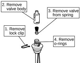
Figure 3-5 Disassembling Mix Pickup Tube
