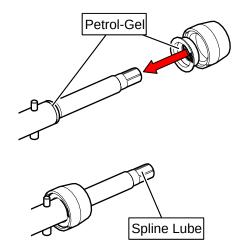
Figure 3-6 Rear Seal Assembly
