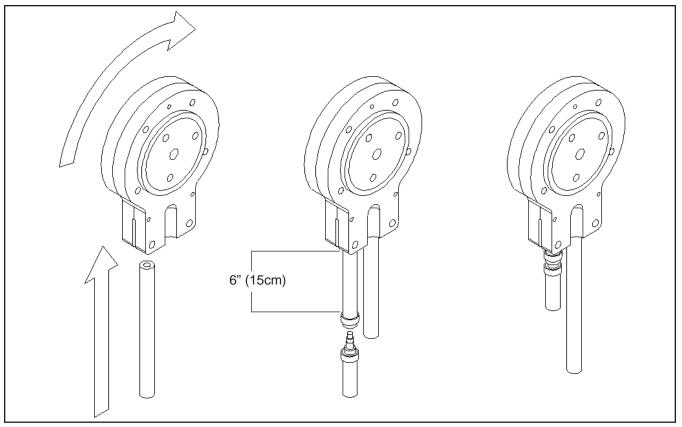
Figure 2-2 Mix Hose Installation
