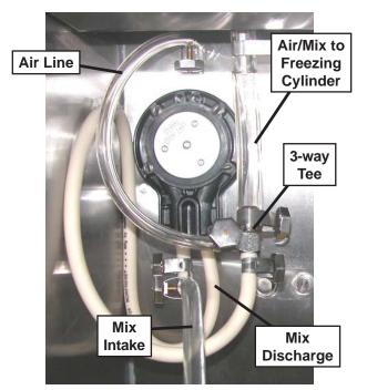
Figure 3-10 Mix Pump Hose Routing
