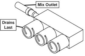
Figure 2-4 BCS Mix Inlet Manifold
