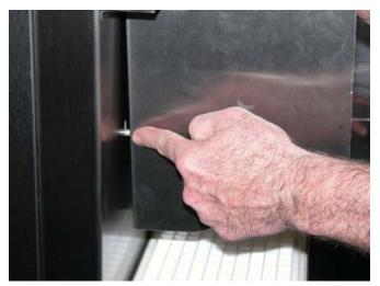
**Figure 3-7 Blender Shroud Pin Alignment**
