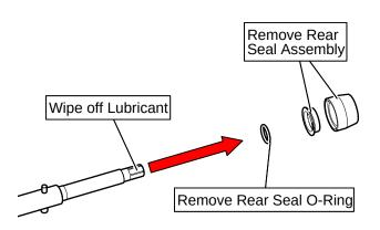
Figure 3-4 Rear Seal Assembly
