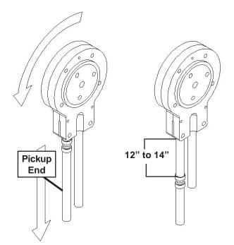
Figure 4-3 Pump Hose Reposition
