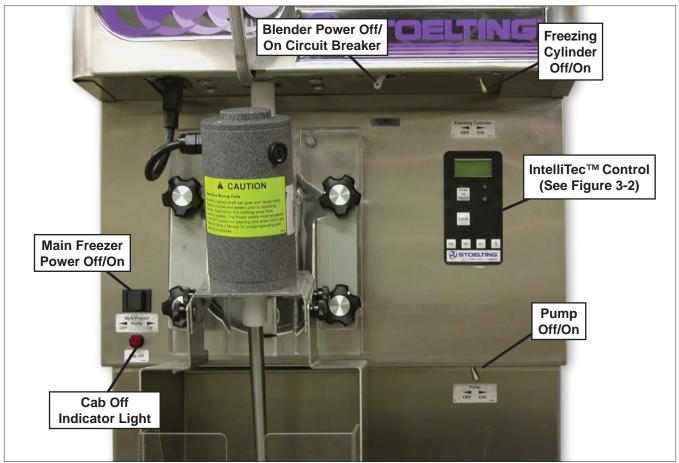
**Figure 3-1 Machine Controls**
