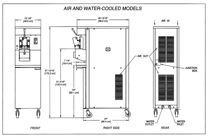
Figure 1-2 Machine Dimensions
