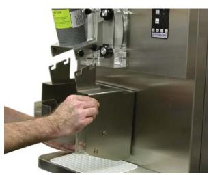
Figure 3-3 Removing Splash Shield Bracket
