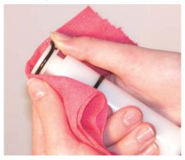
Figure 3-4 Removing O-Ring
