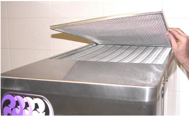
**Figure 2-4 Removing Condenser Filter**
