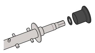
Figure 3-5 Rear Seal Assembly
