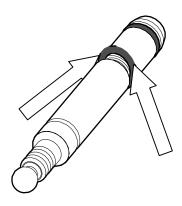
Figure 3-4 Removing O-Ring
