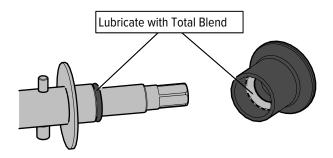
Figure 3-6 Lubricate Rear Seal
