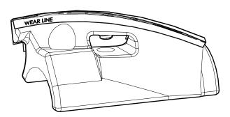
Figure 3-3 Auger Flight Wear
