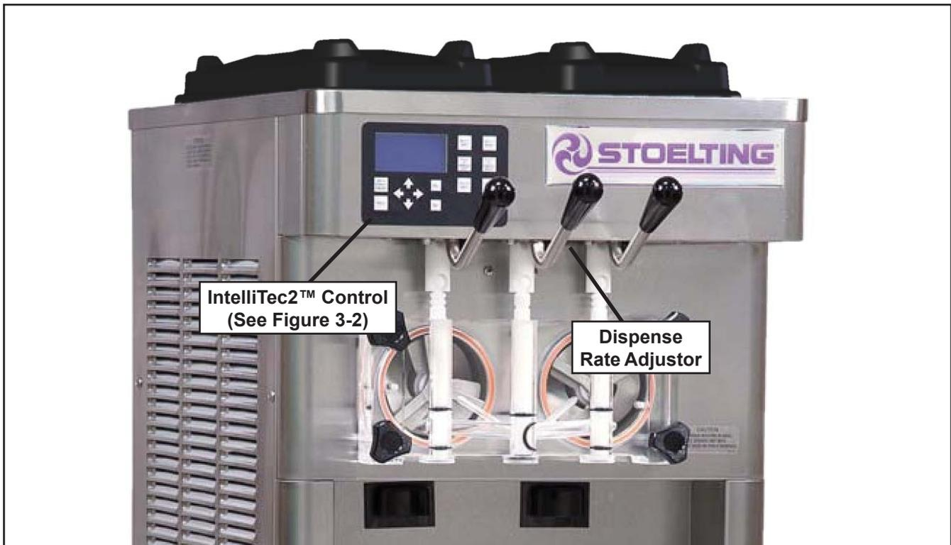
**Figure 3-1 Machine Controls**
