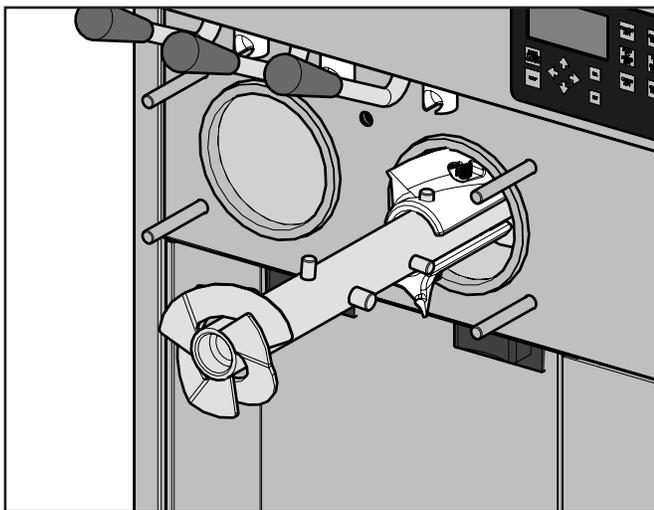
Figure 3-7 Inserting Auger
