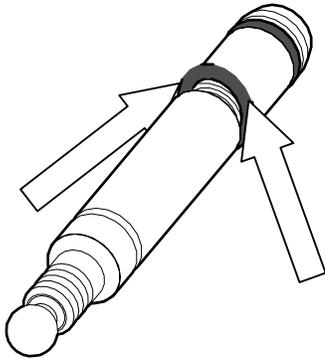
**Figure 3-4 Removing O-Ring**
