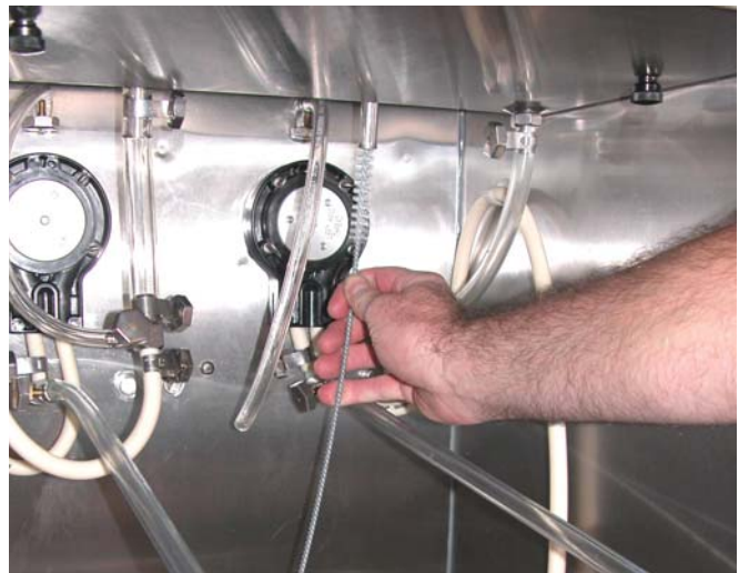
Figure 3-19 Cleaning Feed Tube
