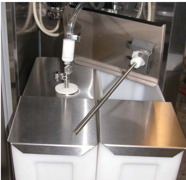
Figure 2-5 Connecting Mix Pick-up Assembly
