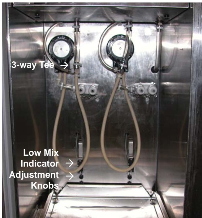
Figure 2-6 Connecting Pump Hose to BCS Manifold
