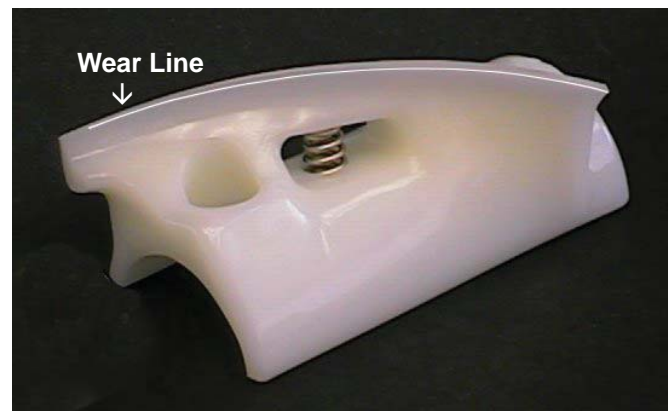
Figure 3-3 Auger Flight Wear
