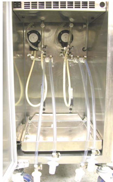
Figure 2-7 Completed BCS Hose Assembly
