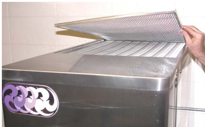
Figure 4-4 Removing Condenser Filter
