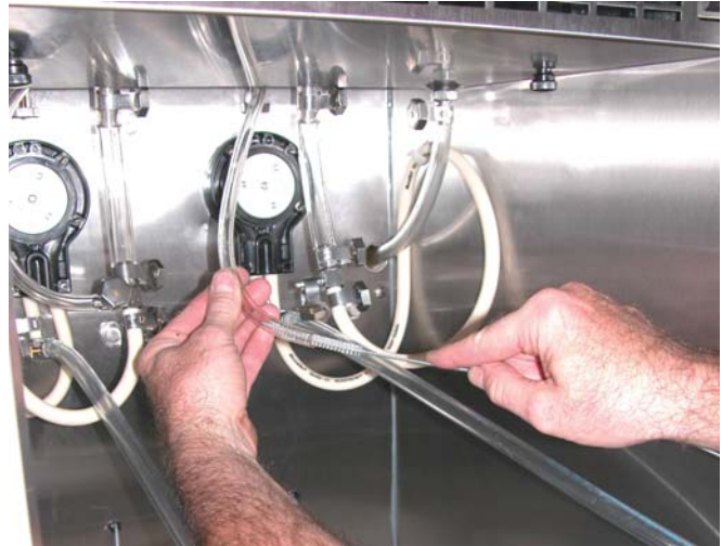
Figure 3-18 Cleaning Air Tube
