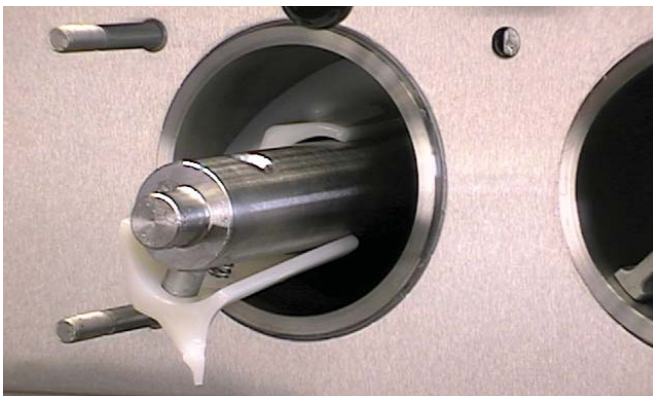
Figure 3-5 Auger Flight Removal
